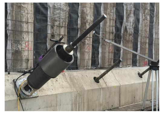
Soil nailing forms part of the comprehensive range of ground engineering processes designed and constructed by Cementation Skanska. Developed in the late 1960's, nailing has since been widely used throughout the world. It is a slope stabilisation process that utilises arrays of fully bonded passive ties installed in the ground. These are usually grouted bars, made from steel, stainless steel or glass fibre.
